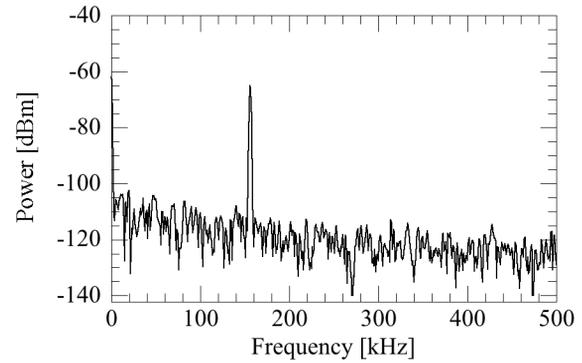
Figure 2: Example of the frequency spectrum of an ion plasma initially perturbed by dipole kicks.
