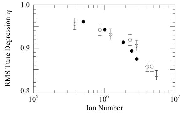
Figure 6: Rms tune depression estimated from the measurement data in Fig. 5 (black dots). For comparison, we have added the previous experimental data (open circles) given in Ref. [13].
