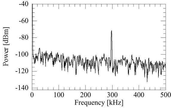
Figure 4: Example of the frequency spectrum of an ion plasma initially perturbed by quadrupole kicks.
