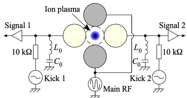
Figure 1: Schematic drawing of the LPT electrodes (cross-sectional view) together with the perturbation driver and image current detector.
