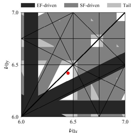
Figure 4: Tune diagram of the J-PARC RCS. The red dot indicates the optimum operating point of the RCS found through considerable experimental effort.
