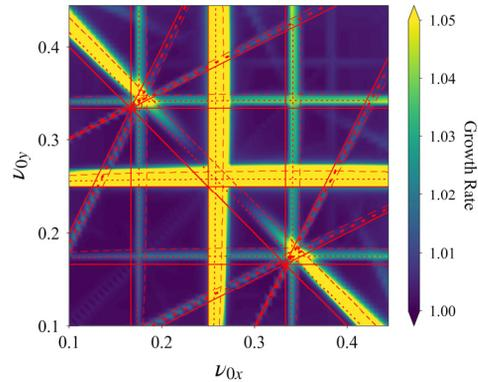
Figure 2: Stop-band distribution obtained from WARP simulations.
