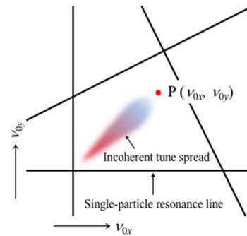
Figure 1: Conventional tune diagram based on the concept of incoherent tune spread.
