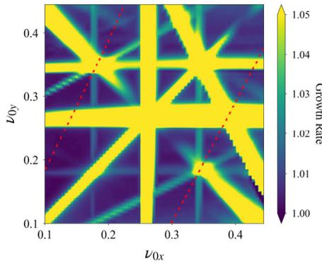
Figure 3: Stop-band distribution obtained from WARP simulations under the condition  $\varepsilon_x / \varepsilon_y = 2$ .
