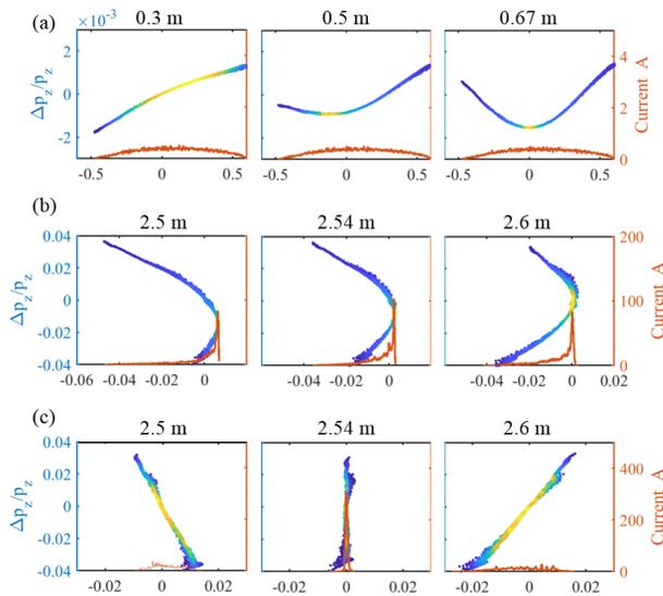
Figure 3: Longitudinal phase space evolution (head to the right). (a) through wake structure. (b) phase space at focus of compression without wake structure. (c) phase space at focus with wake structure.
