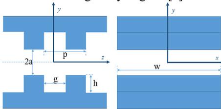
Figure 1: Geometry of a corrugated wakefield structure.
