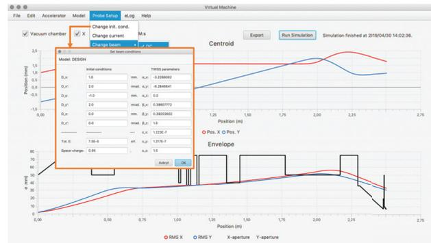
Figure 3: The new OpenXAL VM GUI with the ESS LEBT set up. Functionalities shown are the setting up a beam for simulation and the plots of the simulated DC beam's centroid and envelope functions.
