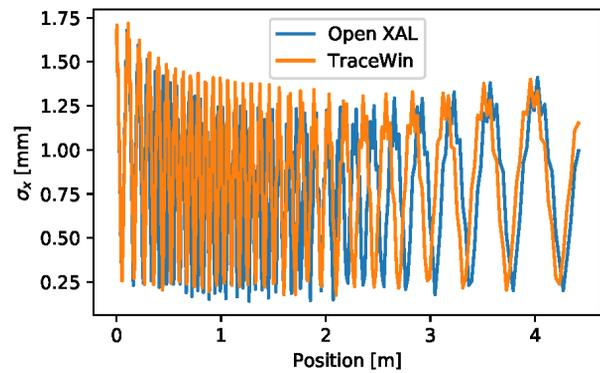
Figure 1: Horizontal beam size in the ESS RFQ simulated using Open XAL (blue) and TraceWin (orange). Initial beam kinetic energy 74.6 keV and no space charge.
