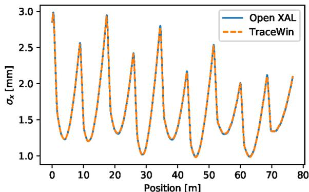
Figure 2: Horizontal beam size in the medium- $\beta$  section (MBL) of the ESS linac simulated using Open XAL (blue) and TraceWin (orange). Initial beam kinetic energy 216.5 MeV and no space charge.
