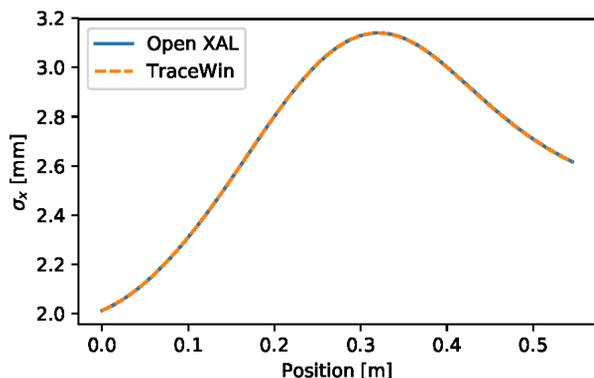
Figure 3: Horizontal beam size in a LEBT solenoid magnet simulated using Open XAL (blue) and TraceWin (orange). Beam kinetic energy 75 keV and no space charge.
