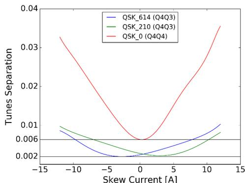
Figure 4: Coupling correction for the Q4Q4 in red and the Q4Q3 optics in blue and green depending on the skew quadrupoles used. The tune separation is plotted versus the skew quadrupole current at the point of the closest approach.
