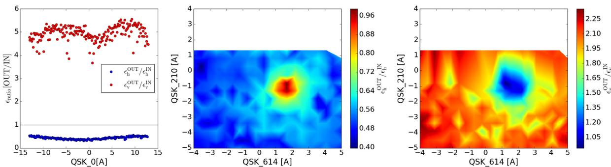
Figure 3: Coupling correction in the PSB. For the Q4Q4 optics (left) the horizontal (blue) and vertical (red) emittance ratios are shown as a function of the powered skew quadrupole current. For the Q4Q3 optics the powered skew quadrupoles current configuration is color coded versus the horizontal (middle) and vertical (right) emittance ratios.
