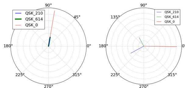
Figure 2: Linear coupling RDTs, phase and amplitude, for the available skew quadrupole magnet families in the PSB, for the Q4Q4 (left) and Q4Q3 (right) optics.
