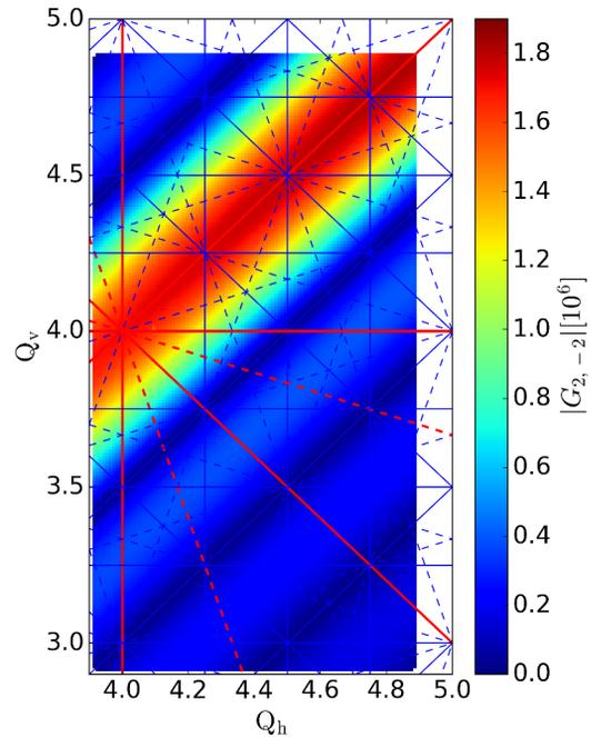
Figure 1: 4<sup>th</sup> order RDT coming from the space charge potential of Gaussian distributions for the PSB lattice. The color code corresponds to the amplitude of the respective driving term at each tune.
