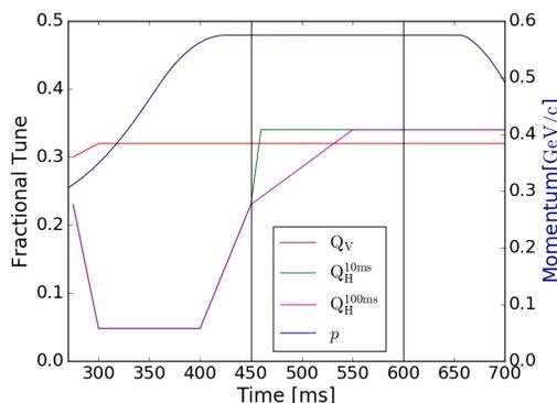
Figure 5: Fractional tunes and momentum along the cycle. The plateau of the momentum corresponds to 160 MeV.
