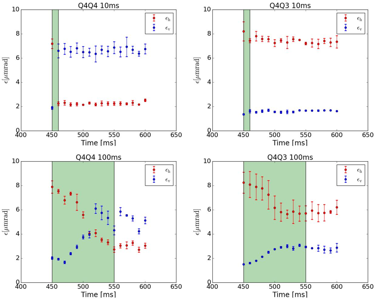
Figure 6: Horizontal (red) and vertical (blue) emittances along the 160 MeV plateau for the Q4Q4 (left) and Q4Q3 (right) optics. The green shaded areas correspond to the time of the tune variation for the resonance crossing, 10 ms (top) and 100 ms (bottom).
