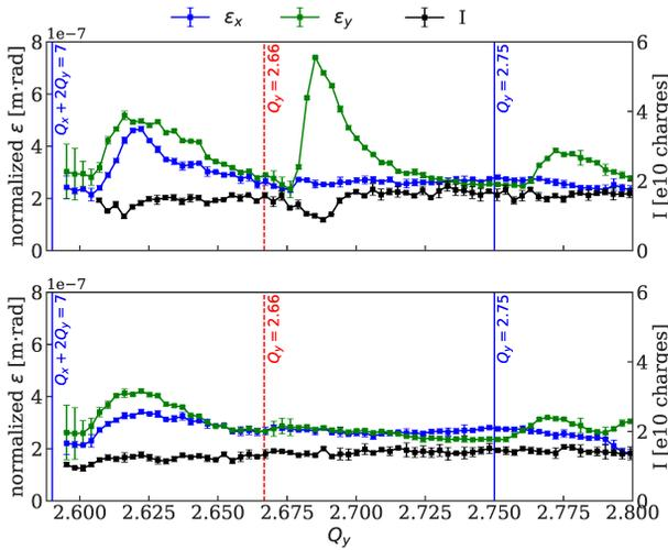
Figure 4: Measured emittances and intensity as a function of the vertical tune at  $t=1000$  ms for the standard machine settings (top) and after compensating the excitation of the skew resonance  $Q_y = 2.66$  by means of a pair of skew sextupoles (bottom).
