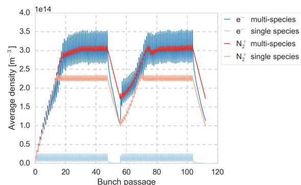
Figure 1: Electron and ion densities during the passage of two bunch trains at LHC injection with a gas density of  $10^{21} N_2/m^3$ , in single-species and multi-species simulations.
