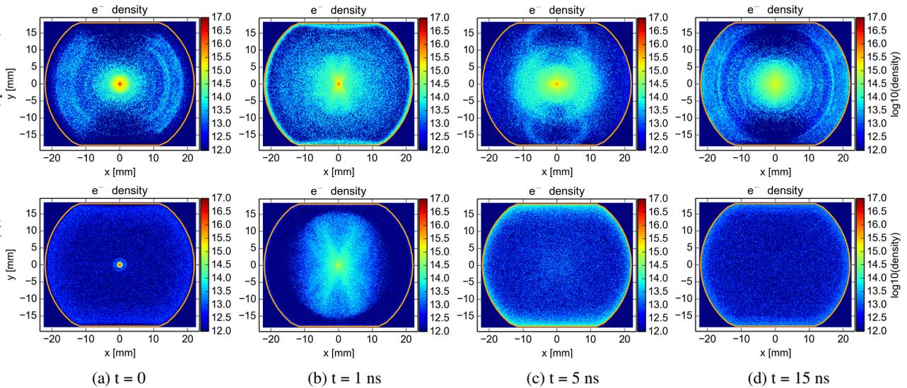
Figure 2: Snapshots of the electron density in the beam chamber during a bunch passage. Images from a multi-species simulation (top), are compared to the equivalent images in a simulation tracking only electrons (bottom). The first image on each row ( $t = 0$ ) is taken during the passage of the centre of the bunch. The bunch length is 1 ns and the bunch spacing 25 ns.
