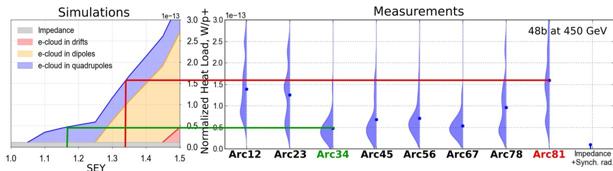
Figure 2: Left: simulated heat load per half-cell as a function of the SEY parameter for two circulating beams at 450 GeV (different contributions are shown in different colors). Right: Corresponding measured heat loads. The curves represent the distribution among half-cells within each arc, the dots represent the average for each arc. The expected load from impedance and synchrotron radiation is shown on the right.
