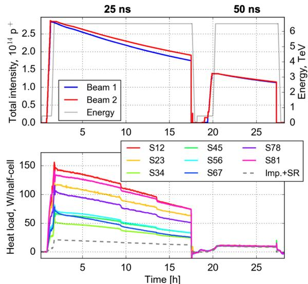
Figure 1: Heat loads (bottom) measured during a regular luminosity fill with 25 ns bunch spacing and during a subsequent test fill with 50 ns bunch spacing, both with  $1.1 \times 10^{11}$  p/bunch. Heat loads are per half-FODO-cell. The total intensity of the corresponding fill is shown on the top figure.
