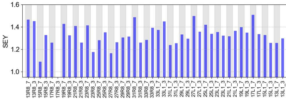
Figure 3: SEY parameter estimated for all cells in one of the sectors showing the highest heat load (S81).
