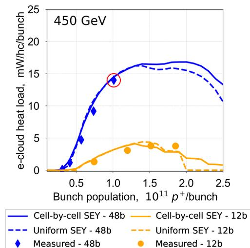
Figure 5: Heat loads at 450 GeV per half-cell as a function of the bunch intensity for one of the sectors showing the highest heat loads (S81). The data point used to infer the SEY is circled in red.
