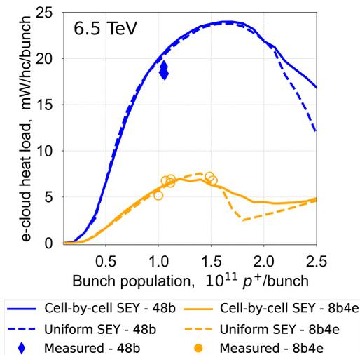
Figure 4: Heat loads per half-cell at 6.5 TeV as a function of the bunch intensity for one of the sectors showing the highest heat load (S81). Simulation results are represented by lines (continuous for the model assuming a different SEY in each half-cell, dashed for the simpler model assuming uniform SEY over the entire arc). Different filling patterns are shown in different colors.
