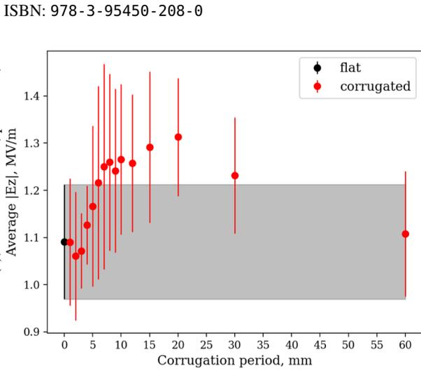
Figure 4: Average accelerating field on axis vs corrugation period.
