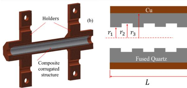
Figure 2: Grated structure a) in its holder sleeve and b) shown schematically.
