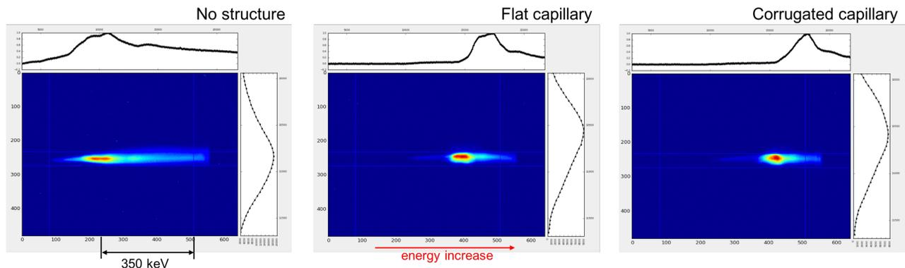
Figure 3: Energy modulation measurements: baseline measurement with no structure (left), flat capillary (middle), corrugated capillary (right).
