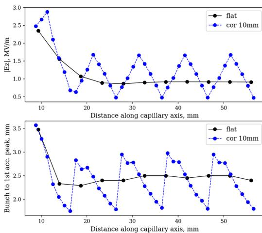
Figure 5: Accelerating field (top) and delay of the peak accelerating field with respect to the drive bunch (bottom) along the structure.
