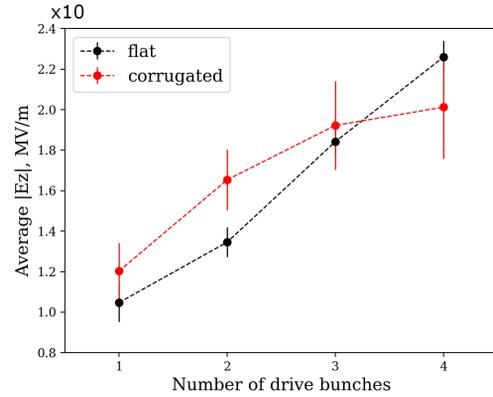
Figure 6: Scaling of the accelerating gradient in case of resonant excitation.
