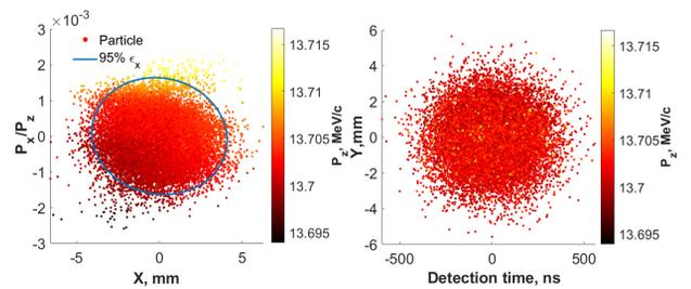
Figure 5: Beam profile at the end of the line. The blue ellipse (left) represents scaled  $\epsilon_x$ . Right plot shows arrival times of particles assuming 0 ns time for the reference momentum particle. An initial bunch length was preserved and has  $\sigma_\tau=150$  ns.
