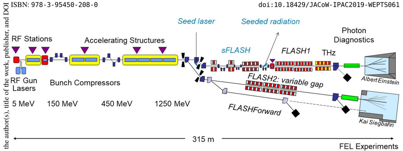
Figure 1: Schematic layout of FLASH user facility. The experiment was performed using the hardware of the seeding experiment sFLASH which is installed in the FLASH1 undulator beamline.
