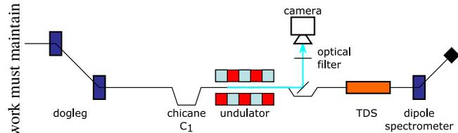
Figure 2: Schematic layout of the experiment. The electron bunches arriving from the dogleg are transported along an approx. 4-m-long beamline segment. After chicane  $C_1$ , the emission from a five-period undulator is extracted from the beamline by an OTR screen and sent to the camera station. The longitudinal phase-space distribution of the bunches can be measured in a combination of transverse-deflecting structure (TDS) and dipole spectrometer.
