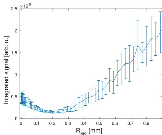
Figure 4: Scan of the longitudinal dispersion  $R_{56}$  with a peak current of 0.4 kA.
