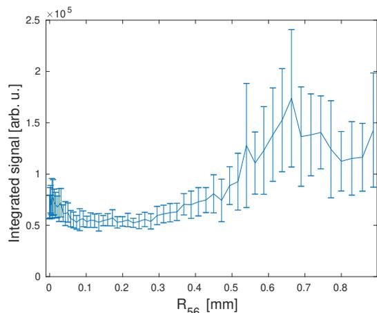
Figure 5: Scan of the longitudinal dispersion  $R_{56}$  with a peak current of 1.0 kA.
