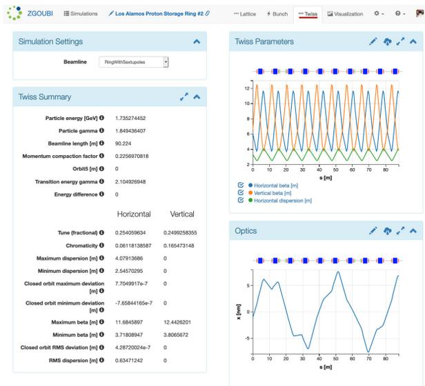
Figure 6: The *Twiss* tab of the Sirepo-Zgoubi interface.
