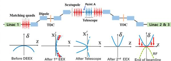
Figure 3: Schematic to explain the principle of DEEX-based energy suppression with a sextupole magnet.
