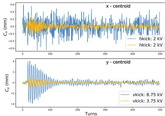
Figure 4: Horizontal and vertical (top and bottom) centroids taken from a BPM immediately after the kickers. The nonlinear element was turned on for this measurement.
