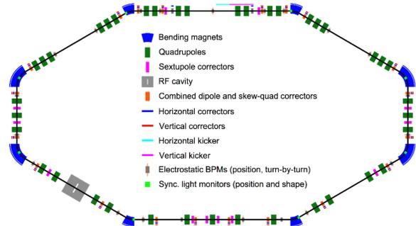
Figure 1: Schematic of IOTA showing position of major elements. The beam is injected in the center of section located at 12 o’clock and passes clockwise through the ring. The nonlinear magnet was placed in the empty section of the first quadrant.
