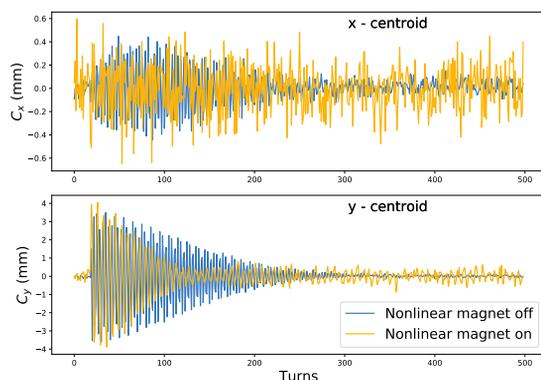
Figure 5: Horizontal and vertical (top and bottom) centroid data, comparing between the nonlinear magnet turned off (blue) and on (yellow).
