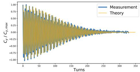
Figure 3: Vertical centroid motion, normalized to peak centroid offset, is shown for measurement with a vertical kick of 11.25 kV. The theoretical line is the plot of Eq. 2
