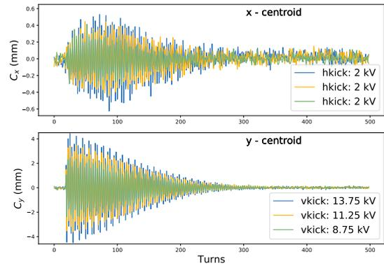
Figure 2: Centroid data for vertical and horizontal (top and bottom) taken from a BPM immediately after the kickers. The nonlinear element was powered down for this measurement.
