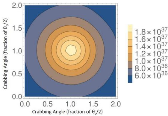
Figure 2: This plot shows the luminosity with both bunches having different crabbing angles.
