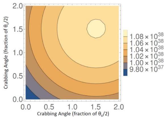
Figure 6: This plot shows the luminosity with both bunches having different crabbing angles for the 800 MHz LHC system.
