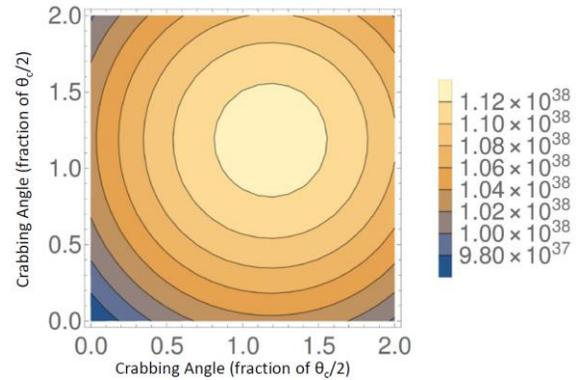
Figure 5: This plot shows the luminosity with both bunches having different crabbing angles for the 400 MHz LHC system.
