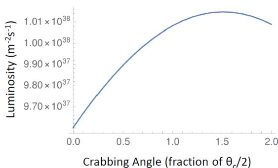
Figure 4: This shows the luminosity of the LHC with 800 MHz of crabbing on one bunch with the other uncrabbed.
