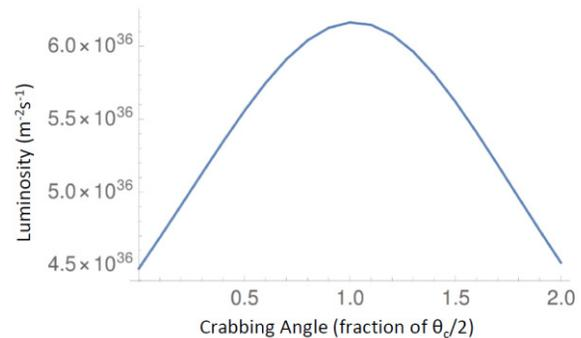
Figure 1: This plot shows the luminosity varying the crabbing angle of one bunch, while leaving the other un-crabbed.
