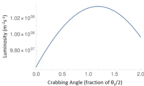
Figure 3: This shows the luminosity of the LHC with 400 MHz of crabbing on one bunch with the other uncrabbed.
