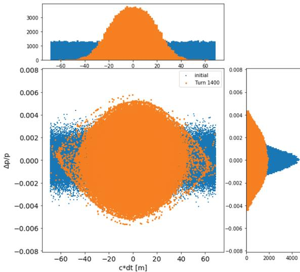
Figure 1: Longitudinal phase space of the beam initially (blue), and after the RF ramp is complete (orange).
