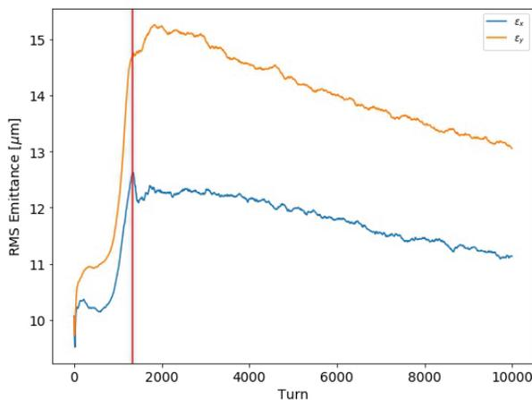
Figure 4: RMS emittance in x (blue) and y (orange) vs turn with an aperture and space charge. The red vertical line corresponds to the turn at which the RF cavity reaches its peak voltage.
