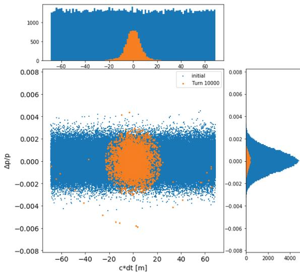
Figure 3:  $\Delta p/p$ - $c \cdot dt$  distribution for the beam initially (blue) and after 10,000 turns (orange) with an aperture and space charge.
