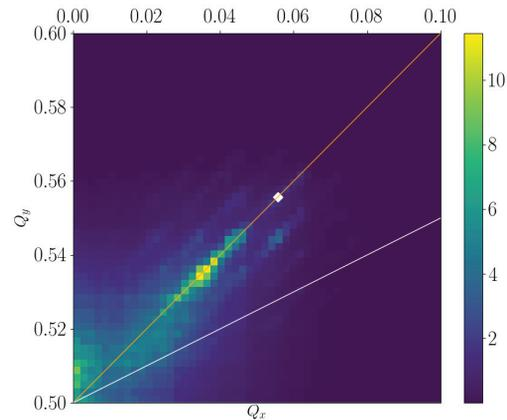
Figure 5: Fractional tune diagram showing the bare lattice tune (white diamond) and space charge tune spread.
