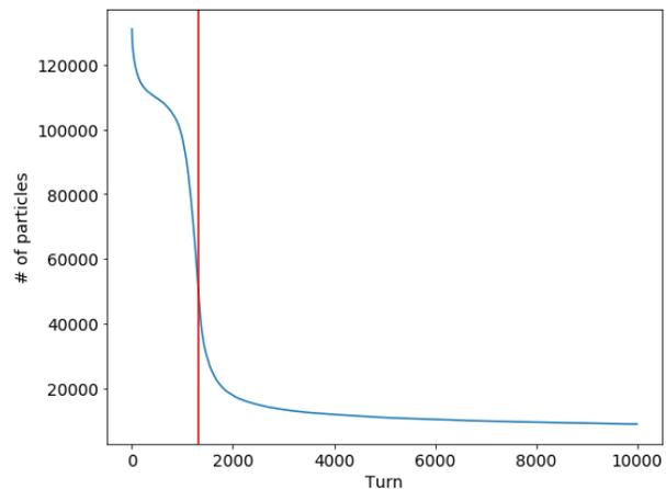
Figure 2: Number of particles vs turn with an aperture and space charge. The red vertical line corresponds to the turn at which the RF cavity reaches its peak voltage.
