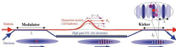
Figure 1: Layout of coherent electron cooler with a high gain free electron laser amplifier.
