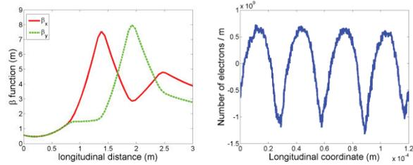
Figure 6: Evolution of electron beam  $\beta$  function (left) and amplified longitudinal density modulation (right) in kicker.
