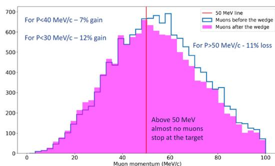
Figure 5: Momentum distributions of muons before and after the wedge. The numbers correspond to 59 MeV/c optimization momentum for the wedge creation and beamline without Collimator 3.
