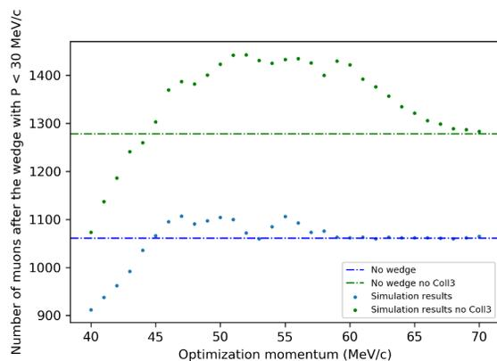
Figure 4: Performance of the C3 wedge with and without the Collimator 3 in obtaining muons with momentum less than 30 MeV/c.
