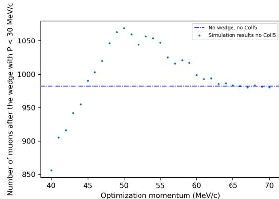
Figure 6: Performance of the C5 wedge without Collimator 5 in obtaining muons with momentum less than 30 MeV/c.
