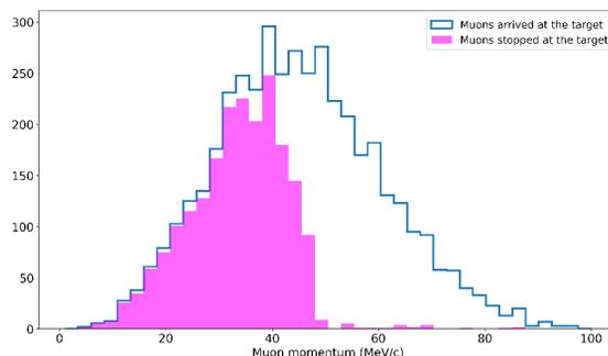
Figure 1: The momentum distribution of muons that arrive at the stopping target and those that are stopped inside the target. The numbers correspond to 200 million protons of initial 800 MeV beam hitting the production target.
