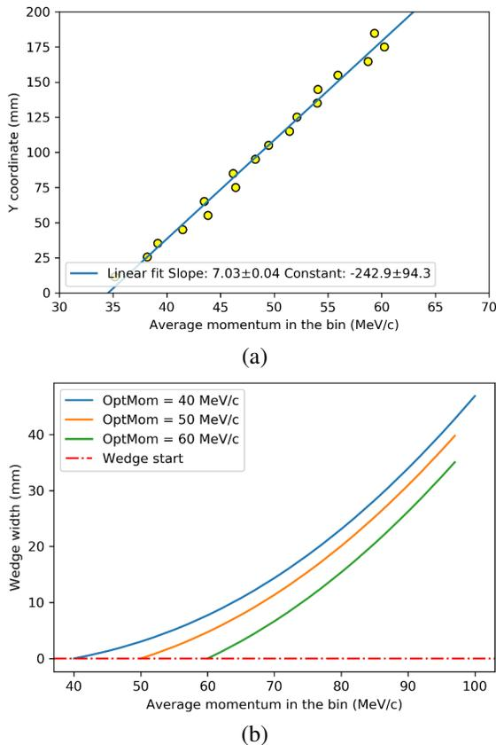
Figure 3: (a) Relationship between the average momentum and the Y coordinate of muons inside the beam in the middle of Collimator 3. (b) Wedge shapes for different optimization momentum values.
