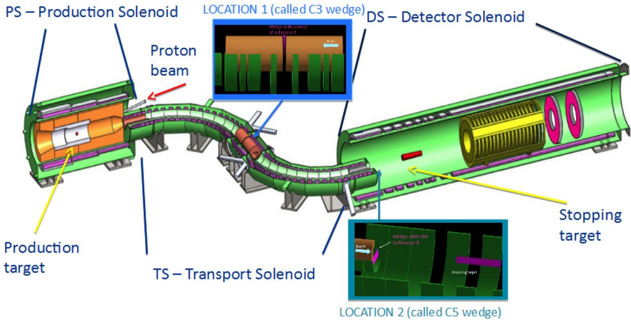
Figure 2: Mu2e apparatus with highlighted tested locations of the wedge absorber.
