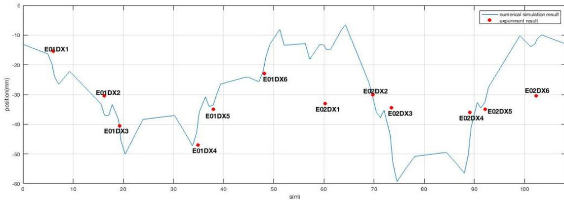
Figure 3: Numerical simulation in ELEGANT and experimental result are shown. The red points are the experimental results and the blue solid line is the ELEGANT simulation. Experiment and simulation are done for an off-momentum particle ( $dp/p=1\%$ ).
