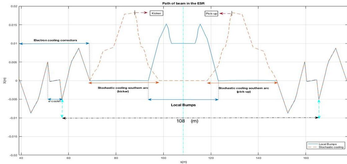
Figure 2: Path of an on-momentum particle in the ESR by simulation.
