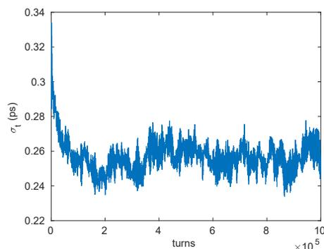
Figure 5: Bunch length tracking of the low- $\alpha_c$  lattice. A bunch of 1000 electrons is tracked for 1,000,000 turns and the bunch length is calculated and recorded.
