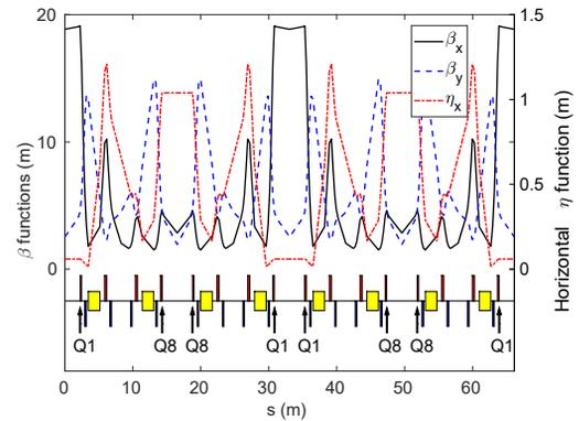
Figure 1: Schematic of the HLS-II linear lattice. There are 32 quadrupoles in the storage ring and they are grouped into 8 families according to lattice symmetry.
