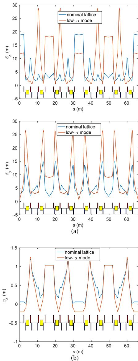
Figure 3: Optical functions for low- $\alpha_c$  lattices and nominal lattice. (a) The horizontal and vertical  $\beta$  functions. (b) The horizontal  $\eta$  function.
