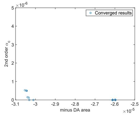
Figure 2: Result of the MOGA optimization of dynamic aperture and second order  $\alpha_c$ . The horizontal axis denotes minus DA area and the vertical axis denotes the second order  $\alpha_c$ .
