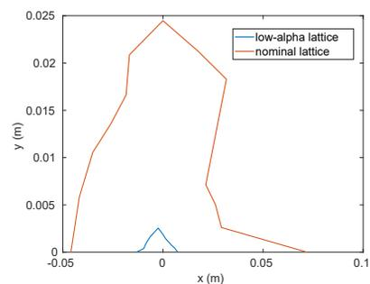
Figure 4: Dynamic aperture of the low- $\alpha_c$  lattice and the nominal lattice.
