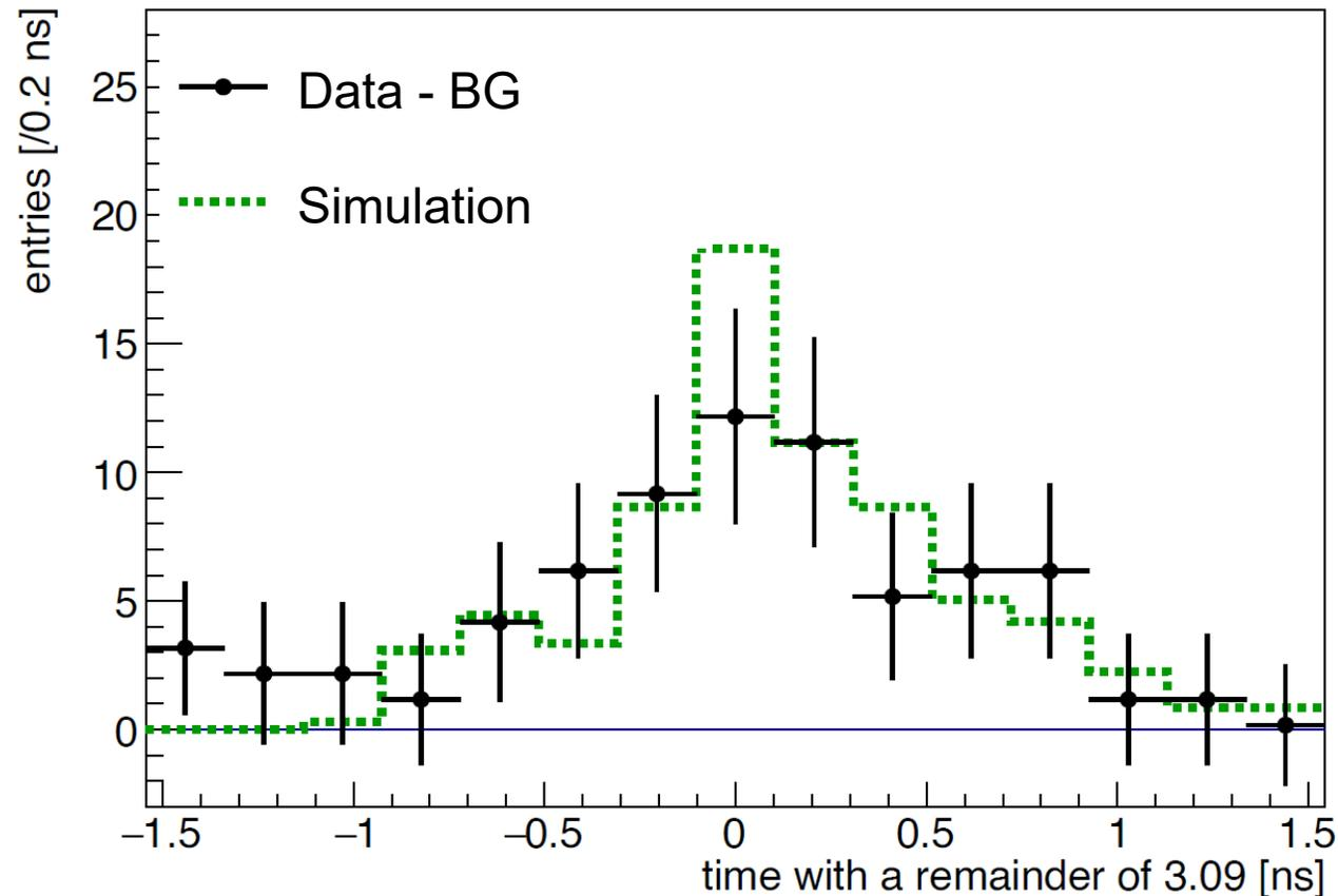
The result of measurement of the bunch size is  $0.54 \pm 0.13$  ns
