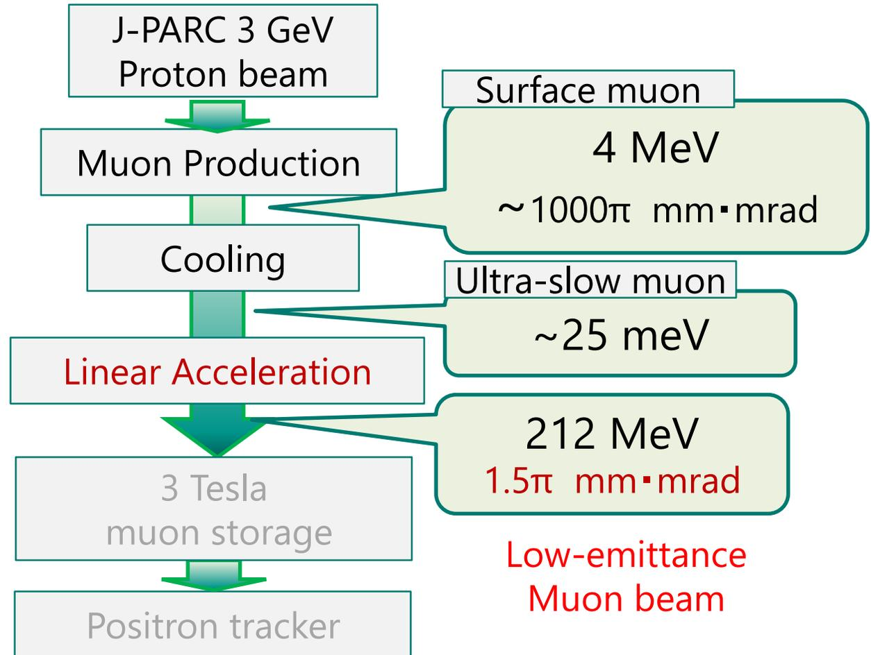
**Muon linac is necessary to provide low-emittance muon beam.**
