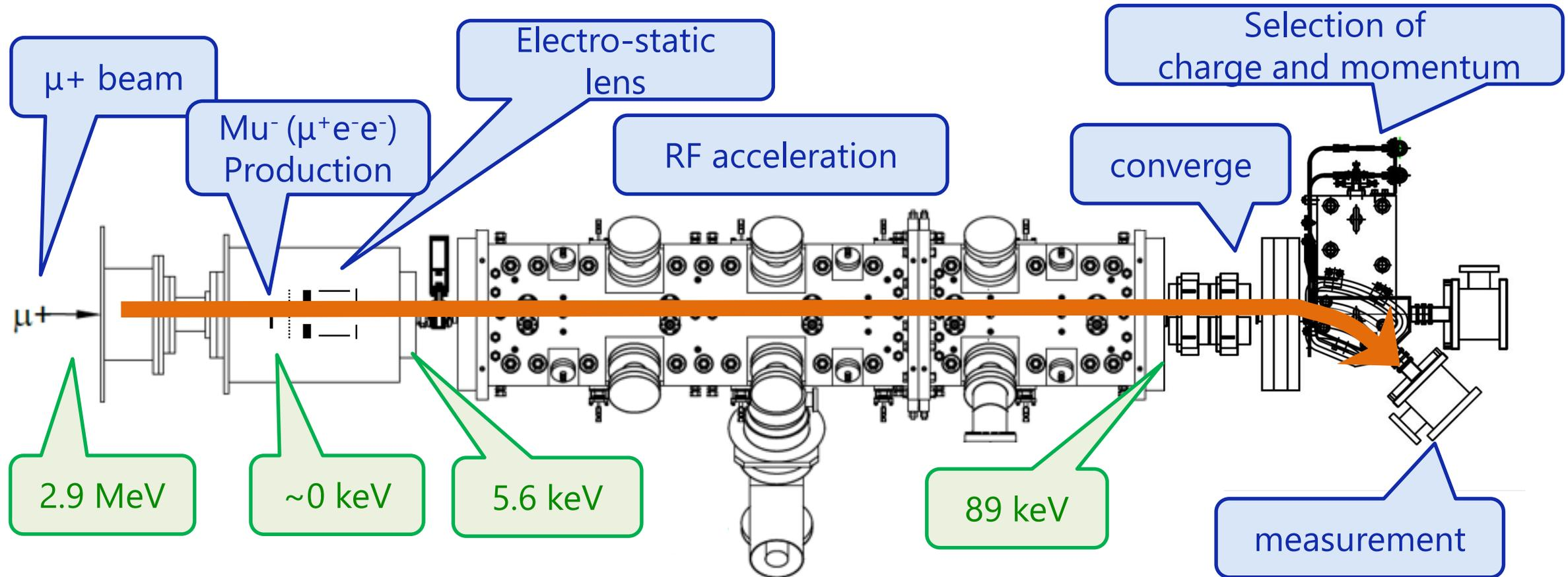
**Produce bunches of the accelerated 89keV Mu<sup>-</sup>( $\mu^+e^-e^-$ )**
