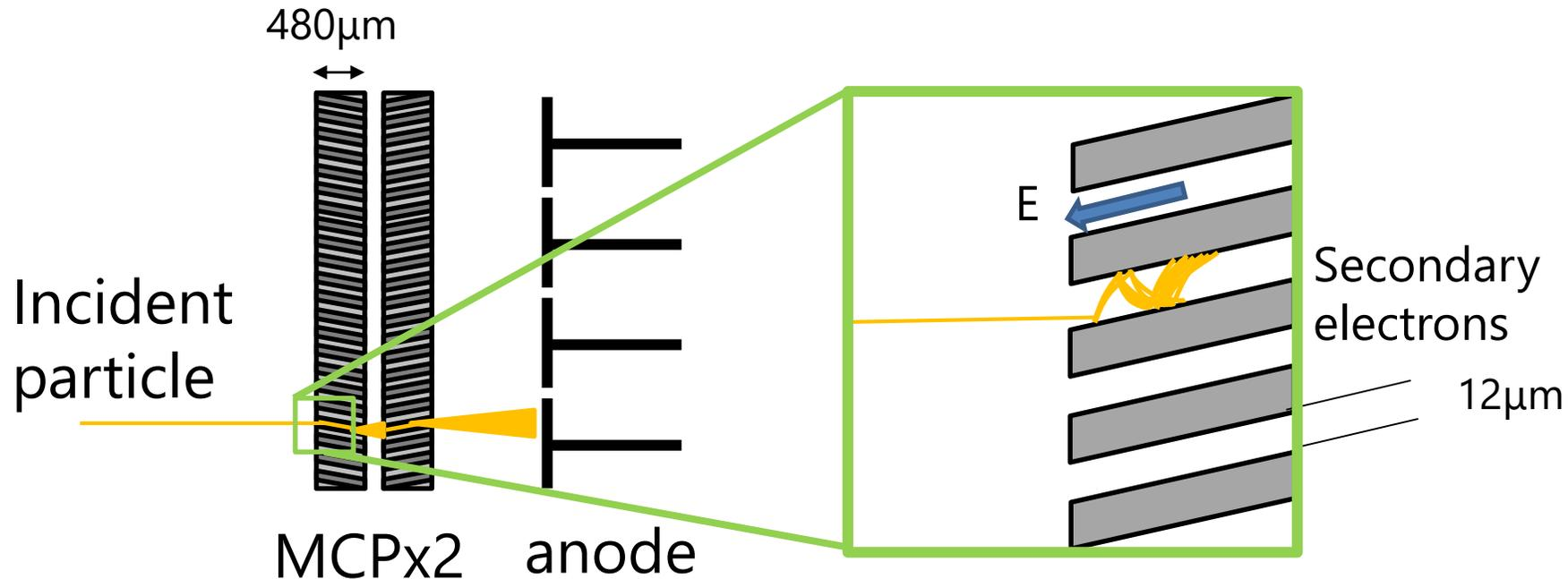
Measure time of muon arrival with high time resolution using MCP
