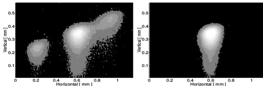
FIG. 14. Synchrotron radiation image of the beam near the  $3\nu_x$  resonance. Left is the situation before the optic is corrected and right is the situation after the optic is corrected. (The plane of the camera is rotated with respect to the plane of the beam.) Also there is a distortion in the light optic in the vertical plane that is responsible for the image’s vertical asymmetry.
