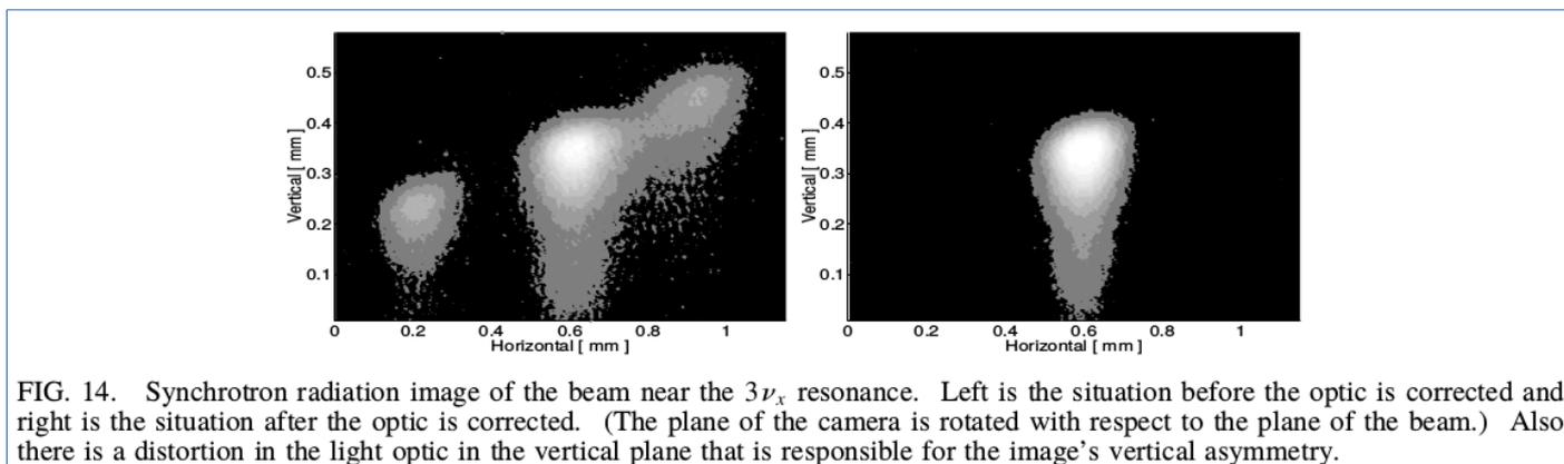
FIG. 14. Synchrotron radiation image of the beam near the  $3\nu_x$  resonance. Left is the situation before the optic is corrected and right is the situation after the optic is corrected. (The plane of the camera is rotated with respect to the plane of the beam.) Also there is a distortion in the light optic in the vertical plane that is responsible for the image’s vertical asymmetry.
