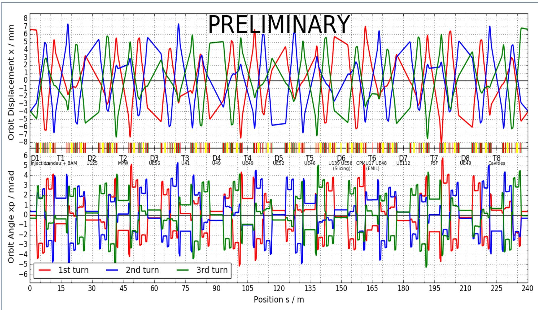
Separation:  $> 10\sigma$  at horizontal source size of  $\sigma_x \sim 300$  mm and divergence of maximal  $\sigma'_x \sim 0.3$  m rad
