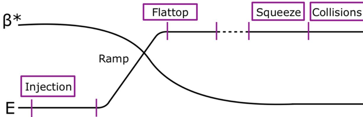
To prepare the machine cycle the collimators must be aligned at all machine states:
