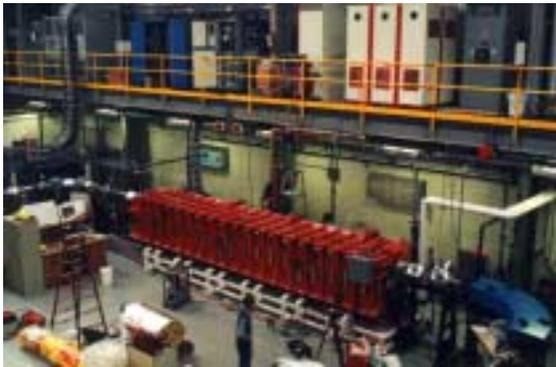
Figure 3. RFQ tank ready for signal level tests
