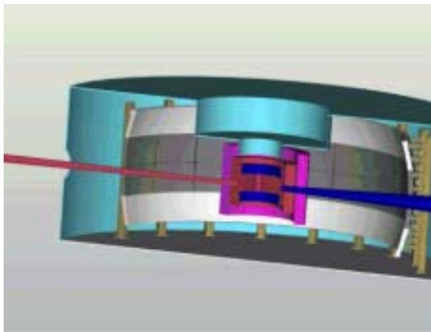
Figure 6: View of the scattering chamber of the backscattering spectrometer. With the analyzer crystals located 2.5 m from the sample, the chamber will have a diameter of approximately 6 m.
