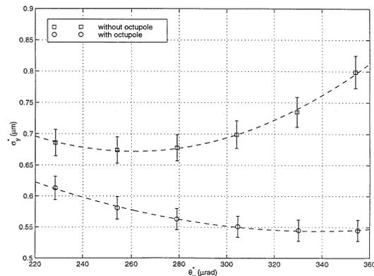
Figure 3: Vertical beam size vs angular divergence at the SLC IP showing the dependence of beam size  $\sigma_y$  on divergence  $\theta_y$ , without (upper) and with octupoles (lower) to cancel higher order aberrations. Both curves are the luminosity-weighted effective beam size.
