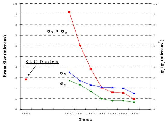
Figure 5: Evolution of beam size at the SLC IP over time from 1991 to 1998 showing  $\sigma_x$  (blue-middle),  $\sigma_y$  (green-lower) and the product  $\sigma_x \sigma_y$  (red-upper). The final beam area was 1/3 of the original design value.
