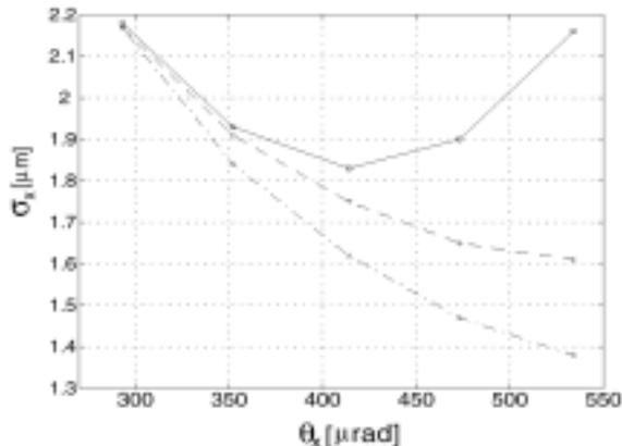
Figure 2: Horizontal beam size vs angular divergence at the SLC IP showing the reduction in beam size for larger  $\theta^*$ . The upper curves are for the 1996 optics, calculated using the RMS beam size (solid) and correct luminosity-weighted effective beam size (dashed). The lower curve (dot-dashed) is for the 1998 optics.
