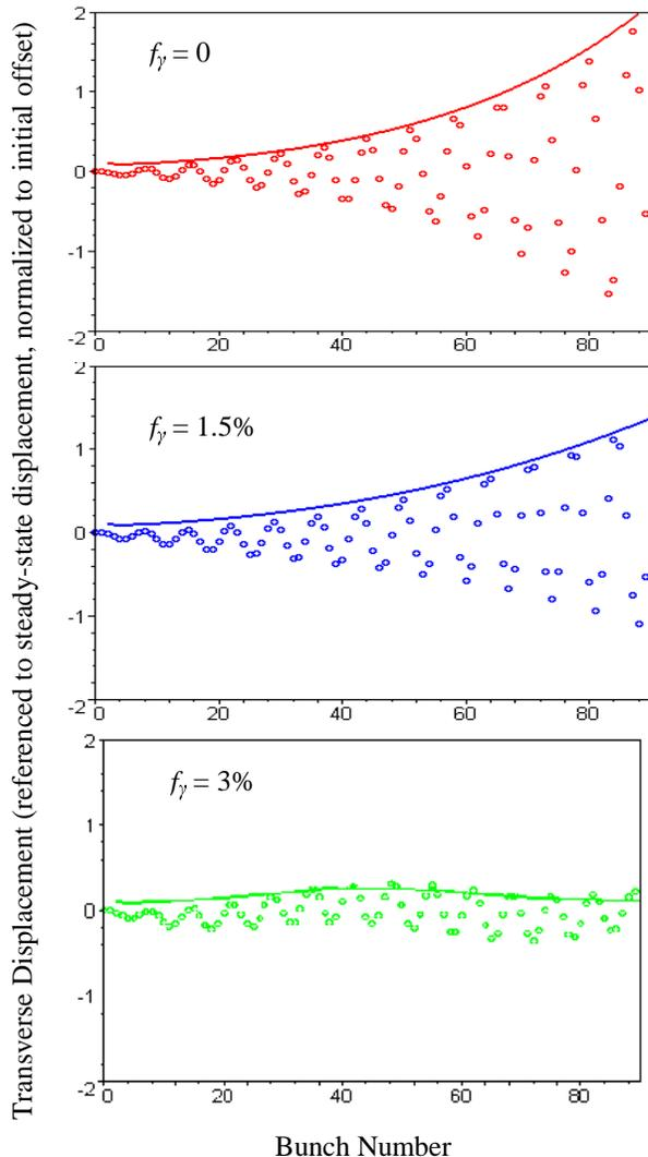
Figure 1: Displacement  $(x_M - x_{SS})/x_0$  vs. bunch number  $M$  at linac exit for Table 1 parameters and  $f_y = 0$  (top), 1.5% (middle), 3% (bottom). Solid curves are analytic solutions for the envelope; circles are numerically calculated displacements.
