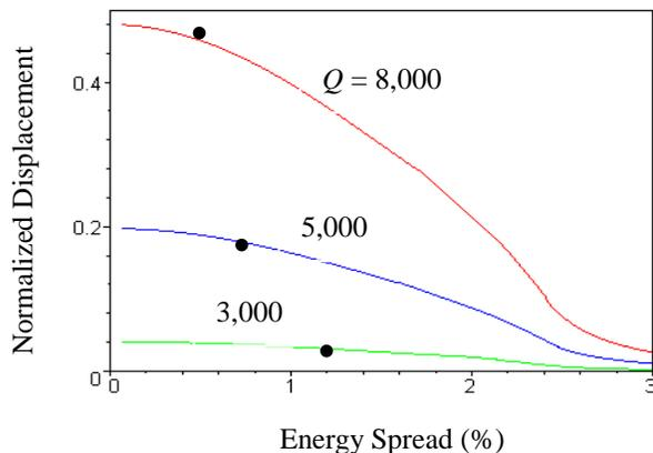
Figure 5: Displacement  $|x_{90}-x_{SS}|/x_0$  of the last bunch  $M=M=90$  at the linac exit versus energy spread  $|f_\gamma|$  for  $Q = 8,000$  (top), 5,000 (middle), 3,000 (bottom). The "effectiveness criterion" is  $|f_\gamma(\%)| > 3,800/Q$ , with the threshold shown for each case (dots).
