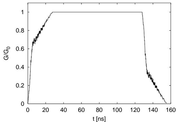
**Figure 3:** Shape of the RF pulse which is produced by the drive beam if delayed switching is applied.
