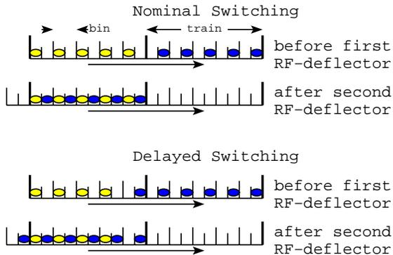
**Figure 2:** The scheme of delayed switching. In this example, each train contains 5 bins (an arbitrary number chosen for better visibility). In the upper case the phase is switched at the nominal time, creating a rectangular pulse. In the lower case the phase switch is delayed to create a ramp.
