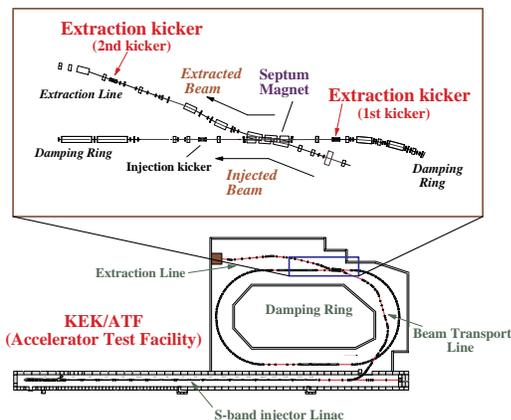
Figure 1: Layout of injection/extraction region of ATF
