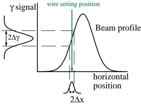
Figure 3: Beam jitter measurement using wire scanner
