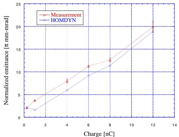
Figure 3. Minimum normalized emittance at the exit of the 9-cell versus the charge per bunch.
