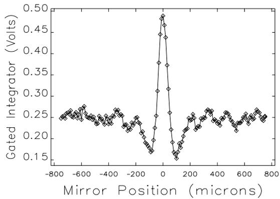
Figure 5: Autocorrelation of the gated integrator CTR signal.
