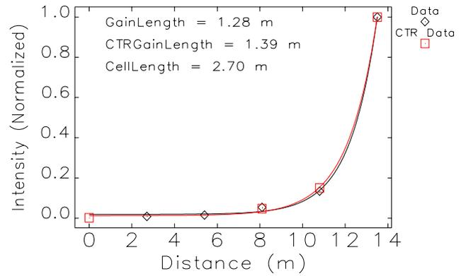
Figure 8: SASE gain measured at undulator diagnostics stations.
