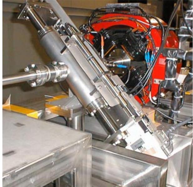
Fig.1: Wire scanner chamber in ATF extraction line.
