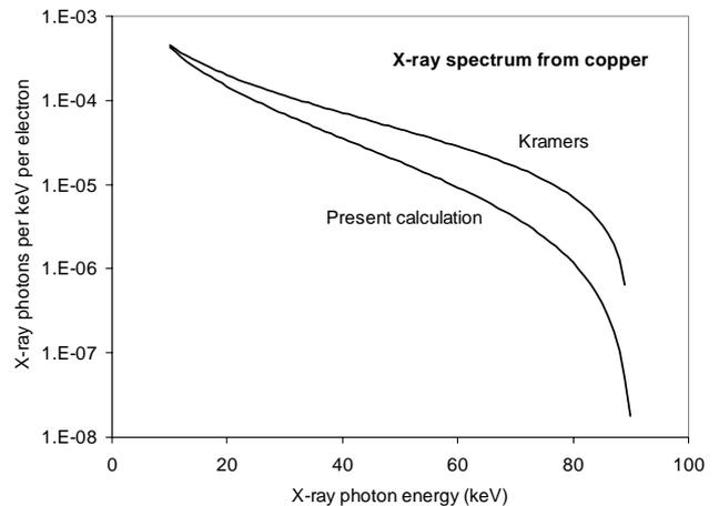
Figure 1 Comparison of X-ray spectra calculations
