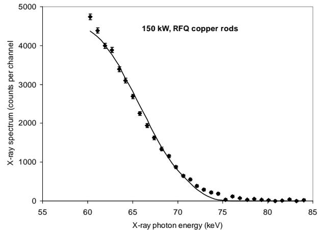
Figure 2 Comparison of measured and calculated X-ray spectra
