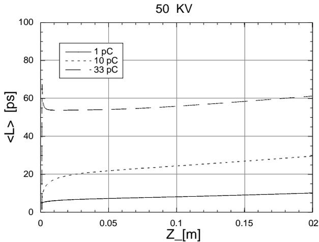
Figure 6: Evolution of bunch length from cathode to deflector by 50 kV voltage applied. Maximum extracted charge in this case is 33 pC.
