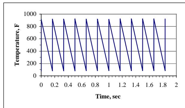
Figure 3: Predicted scraper temperatures
