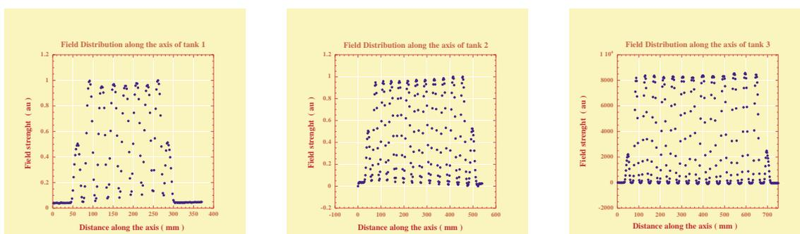
Fig. 3 Electric field distribution of the IH tank 1, 2 and 3.
