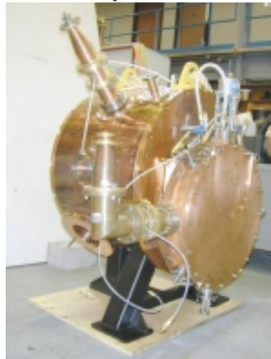
Fig. 1 Photograph of tank2 and buncher assembly being prepared for RF power test. The buncher is the small cavity in front of the tank.
