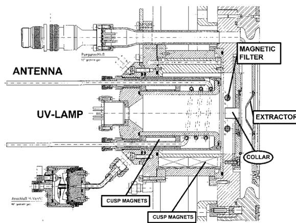
Figure 1: The DESY volume source with an rf coil shielded by Al<sub>2</sub>O<sub>3</sub> ceramic.
