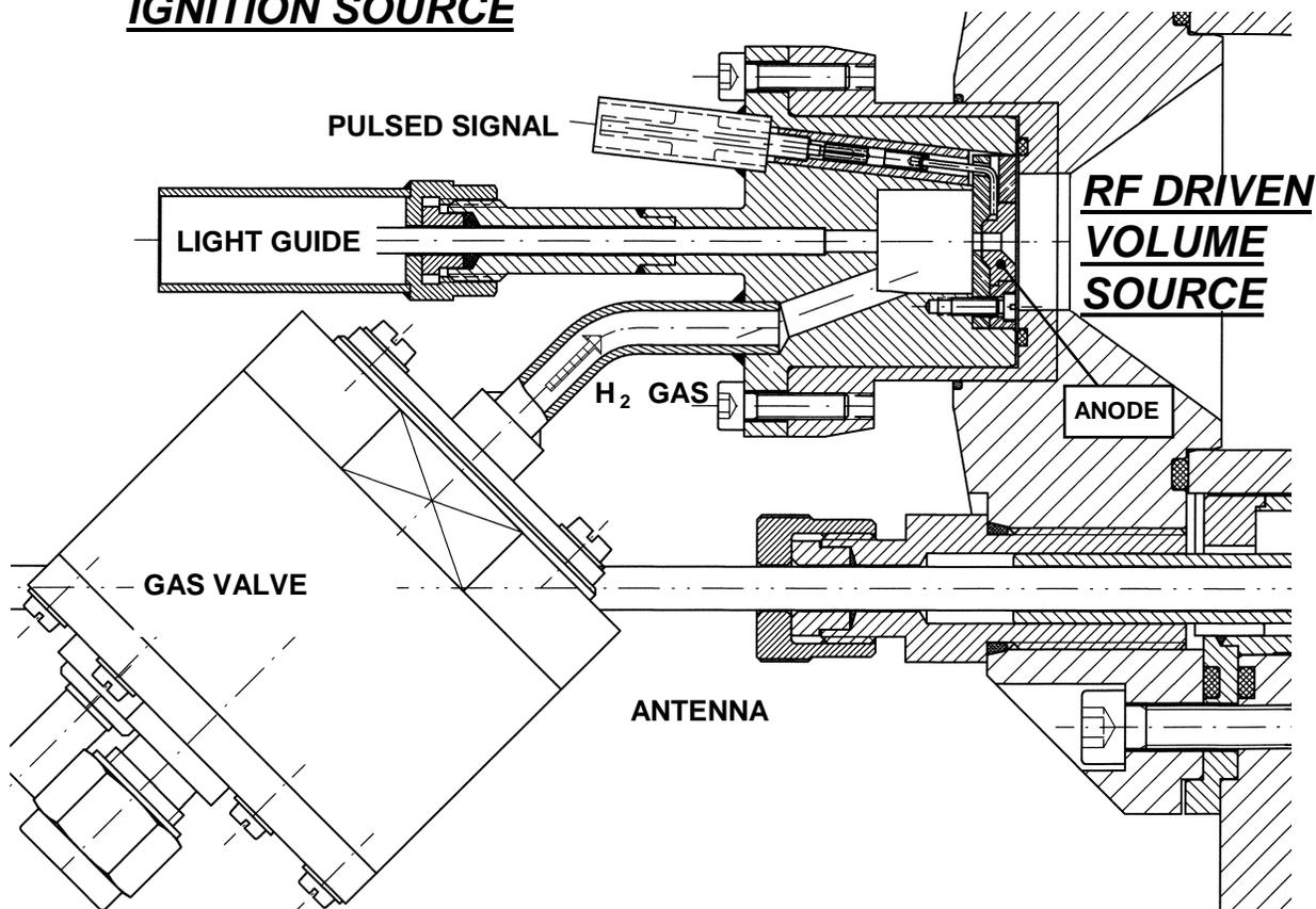
Figure 2: The DESY ignition source mounted to the RF - driven volume source together with the gas valve
