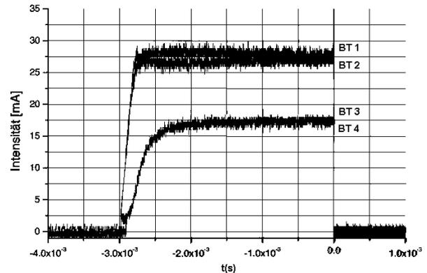
Fig. 4 Beam transformer signals along the beam line.
