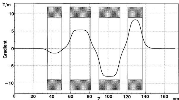
Fig. 6 Measured quadrupole quartet field distribution
