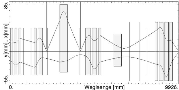
Fig. 2 Transverse envelope of a zero current beam
