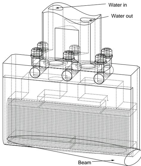
Figure 3: Chopper Target
