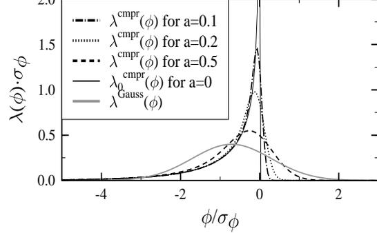
Figure 2: Longitudinal charge distribution for a compressed bunch with intrinsic width described by  $a$ , compared with a Gaussian distribution. All the distributions here have the same angular rms size  $\sigma_\phi$ .
