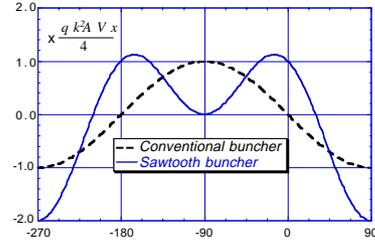
Fig. 5 RF defocusing terms for the approximated sawtooth function and the conventional sine function.
