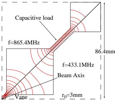
Fig. 7 An example of harmonic cavity for a four-vane DFQ. Beam axis is bottom left.
