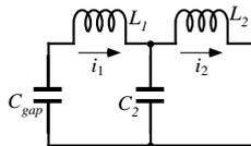
Fig. 9 The equivalent circuit for the DFQ
