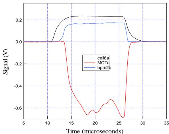
Figure 3: Plots of RF field in the linac (top trace), electron bunch charge (middle trace) and HgCdTe detector signal (bottom trace) as a function of time. The infrared power impinging on the HgCdTe detector has been strongly attenuated.
