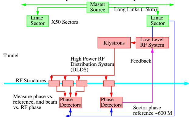
Figure 1 Overall Layout of the Distribution System
