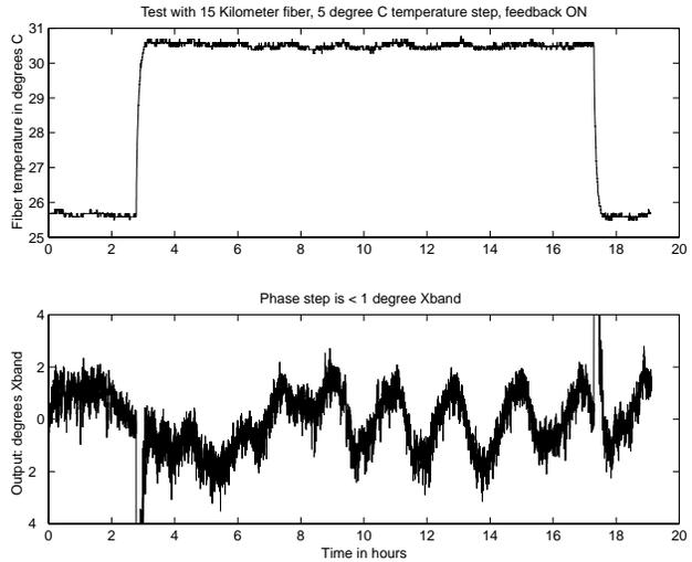
Figure 5: Phase stability for a 5 °C temperature step.
