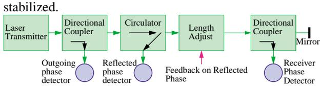
Figure 2: Long Link Schematic
