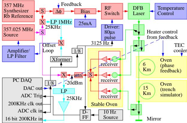
Figure 4: Phase Stabilization Test System
