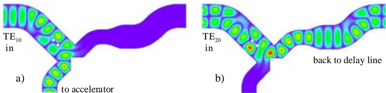
Figure 3: Extractor with simulated electric field plots illustrating a) extraction of the  $TE_{10}$  mode and b) passing the  $TE_{20}$  mode. For the latter, a “jog converter” attached to the through port after a width taper restores the mode and brings the port back in line with the delay line. Power flow is from the left port.
