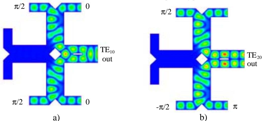
Figure 2: Example Cross Potent Launcher with simulated electric field plots illustrating launching a) TE<sub>10</sub> and b) TE<sub>20</sub> in the right overmoded rectangular port with the indicated relative phases for four equal amplitude inputs. Alternate phasings of the inputs send the power to either of the left ports.
