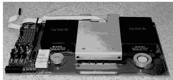
Figure 5. PC Board Core Driver circuit
