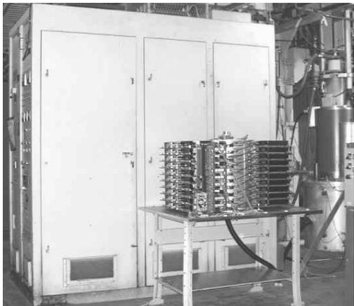
Figure 8. Table Top Induction Modulator
