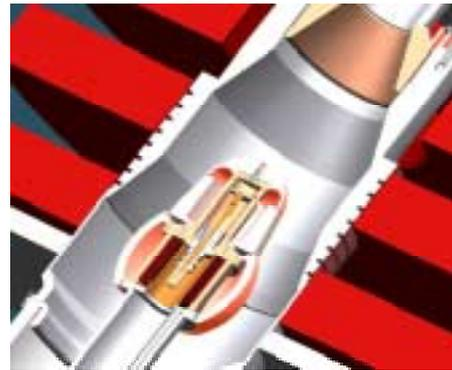
Fig. 3. Magnetron injection gun sectioned view
