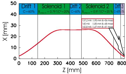
Figure 7: Schematic drawing of the magnetic LEPT for IFMIF including beam envelope for 140 mA.
