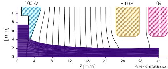
Fig. 1 : Geometry used for simulation of the ion extraction. The potential distribution and beam trajectories (nominal current 140 mA) are shown.
