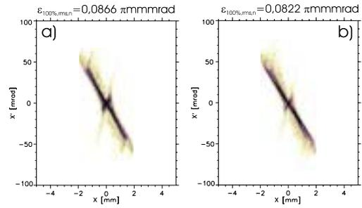
Figure 9 : Time integrated emittance gained from simulations of beam transport using entrance emittances according to fig. 1(a)  $f_{\text{noise}} \approx 100$  kHz, (b)  $f_{\text{noise}} \approx 500$  MHz).
