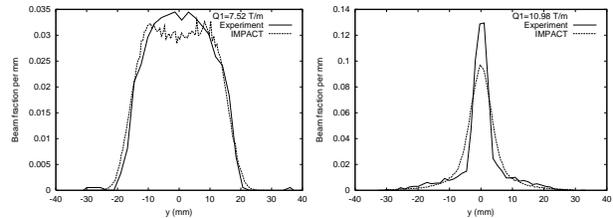
Figure 2: Profile at wire scanner for  $y$  scan with Q1=7.5 T/m (left) and Q1=11 T/m (right). Solid curve is the experimental measurement and the dashed curve is the IMPACT simulation using the LINAC-fit beam as input.
