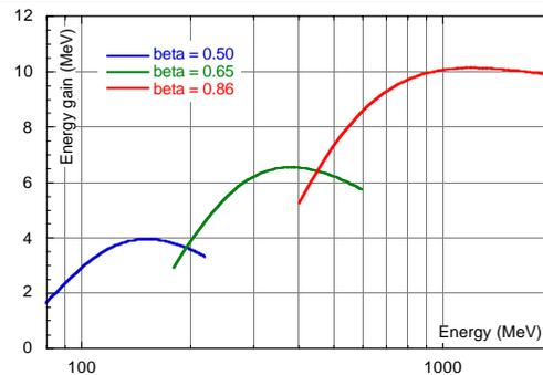
Figure 1: Energy gain for the 3 cavity types.
